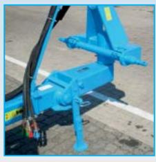
The stand is multiple heights adjusting, which guarantees an optimal position of the headstock for coupling and uncoupling of the tractor. The stand can be quickly moved from parking into transport position by readjustment of a spring-loaded pin.
