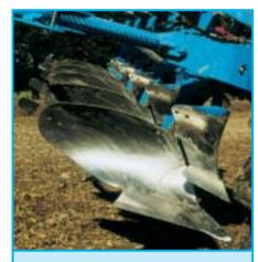
The frog is hardened and tempered and thus immensely strong. The plough body is adjustable for pitch and thus always allows good entry into the soil. The smooth transition from share to mould-board and the low-resistance shape make the plough even lighter to pull.
