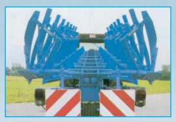
For fast and safe transport on roads, the plough will be turned until the plough bodies are parallel to the ground (the butterfly position) and locked by means of two lock valves. Now the plough can be towed as easily as a single axle, articulated trailer. So the tractor and the plough are protected against overload.
