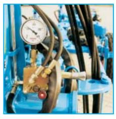
The adjustment range, controlled by a handwheel on the control block, is between 50 and 140 bar.
