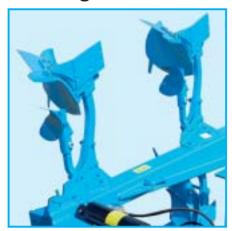
Plough bodies fitted laterally to the frame and the unique shape of the legs give exceptional large clearances between the plough bodies. So clogging will be avoided also when working with narrow working widths.
