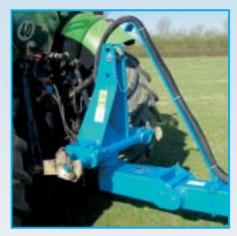
The category II or III one-piece drawbar is elastic and absorbs high shock loads and protects the tractor and plough headstock.
