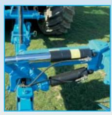
Two telescopic rams turn the plough smoothly and positively through 180 degrees.
