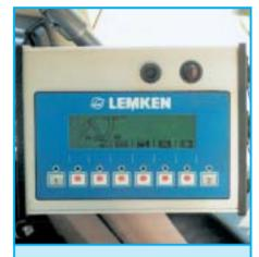
The sensing system warns the tractor driver via a control terminal with optical and acoustic signals when freely-programmable limits to the plough line are neared or exceeded.
