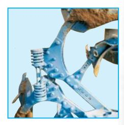
With EuroDiamant and Vari-Diamant ploughs with automatic overload safety systems the skimmers can be moved along the beams. Working depth adjustment is made with pins and therefore no-tool are required. For the ability to adjust the angle, round stalks are available.
