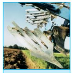
The slats of the slatted body are of thick, completely hardened, special steel and individually exchangeable. The securing bolts are deeply countersunk to guarantee that slats still remain firmly attached after extremely long usage. Slatted bodies and normal mouldboards are based on the same frog.
