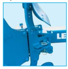
The EuroDiamant and the Vari-Diamant with shear bolt device are available with individual quick adjustment system for the skimmer angle. This allows precise aiming of the trash flow.
