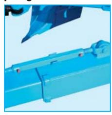
The front-furrow width can be set by adjusting a turnbuckle. An hydraulic option from the tractor seat is available.
