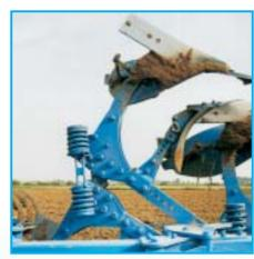
Neither at trip or re-entry does any significant amount of frictional resistance occur at the spacing roller between the tandem beams. This means that force losses at re-entry of a plough body are reduced to a minimum. The result is a consistent tripping characteristic: gentle and shock-free followed by powerful, rapid re-entry of the plough body.
