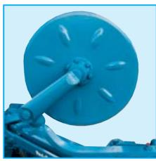
The plain 500 mm diameter disc coulters feature side mouldings which encourage the disc to keep revolving even when cutting through a lot of organic material. Depth adjustment is through vertical swivelling of each coulter arm which is screw-locked into a toothed bracket. The adjustable bearings, fitted with plain side towards the ploughed land, are double sealed against dirt ingress.
