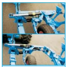
Depending on type of tractor and tyres, it is possible to change this semi-mounted reversible plough from onland to in-furrow mode just using the hydraulics from the tractor seat. The front support wheel for onland ploughing runs within the plough frame thus giving the large clearance necessary when reversing the plough. For in-furrow ploughing, this wheel is locked in the mid-position so there's no need to dismantle it.
