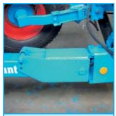
The horizontal draught point can be easily adjusted via a simple bolt setting. This allows precise load transfer onto the rear axle of the tractor. Where a tracklayer is used the draught point for a consistent loading on the tracks is set far down. The system means optimum draught transfer is achievable for all tractor types with resultant minimum wheel or track slip.
