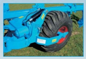
The very large dimensioned depth wheel minimises the soil pressure during work and ensures the required safety when driving on roads.
