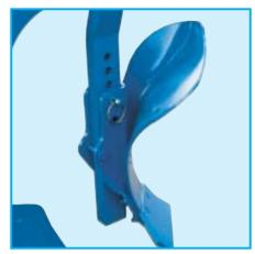
Fitting the skimmer onto a flat stalk avoids danger of them twisting. All shares and mouldboard variants can be exchanged without any problem because the frog is the same. For ploughing without skimmers these can be quickly removed because only two bolts have to be loosened in each case.
