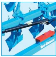
The plates for the leg pivot bracket are bolted to the frame. This gives very positive location, great strength and long life.
