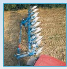
The large clearance between turnover mechanism and tractor enables the tractor to turn sharply = 90 degrees on headlands. By means of turning the plough frame, the depth wheel is steered automatically.
