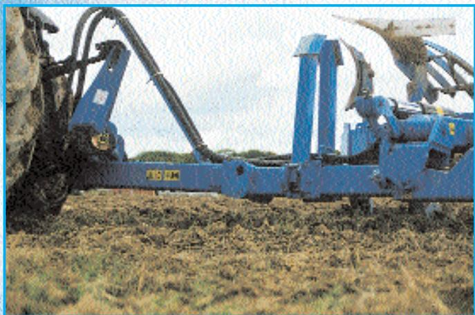
The one-piece shock-absorbing category III or IV plough drawbar is simply adjustable for height. It protects tractor and plough headstock through absorbing larger shock loads. The headstock axle material is well-tempered. The axle runs on roller bearings and is easily lubricated. All this means great strength and long working life.
