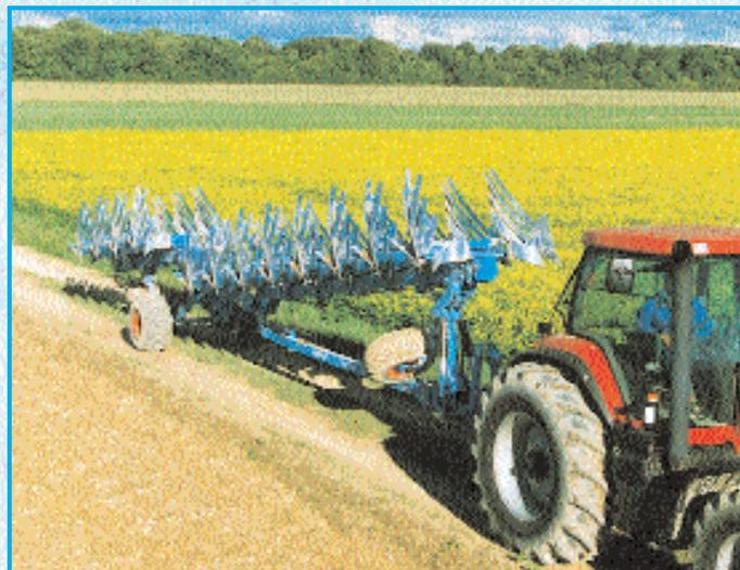
The generously dimensioned wheels for the semi-mounted plough minimise ground pressure during work and offer the required security in road transport. The wheels are fitted with 38x20.0-16,1 or 405/70 R 20 tyres.
