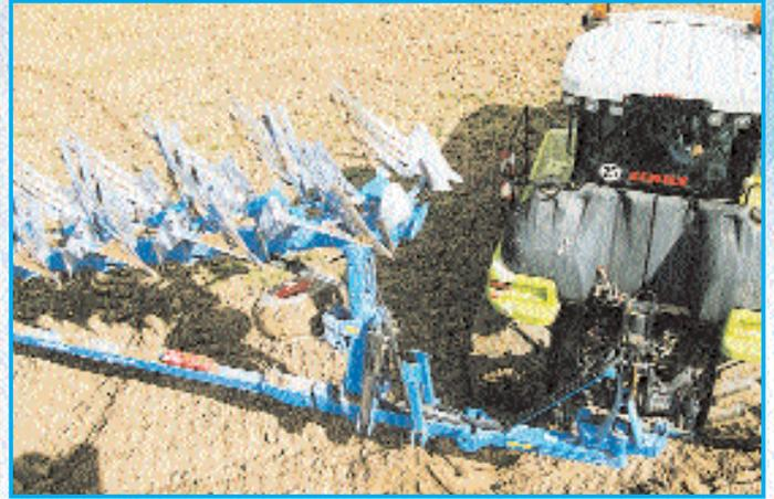
A large amount of free space between tractor and headstock enables turning angles of up to 90°, increasing manoeuvrability on headlands and substantially simplifying ploughing operations with dual-wheeled tractors. Axle of turnover mechanism and wheel axle co-ordinate well for quick turns simply carried out with highest stability, even on narrow headlands in hilly fields.
