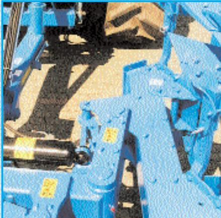
The semi-mounted reversible Vari-Titan plough can be rapidly changed from on-land to in-furrow mode. The adjustment system on the front turning mechanism allows on-land ploughing with tractors up to 3.80 m wide.
