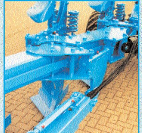
The robust square-tube frame of micro-alloy fine-grained 10 mm steel is notable for its light weight, superior strength and long working life. The frame plates for the mounting of the adjustment brackets are bolted to the frame giving exact precision and long-term solidity.
