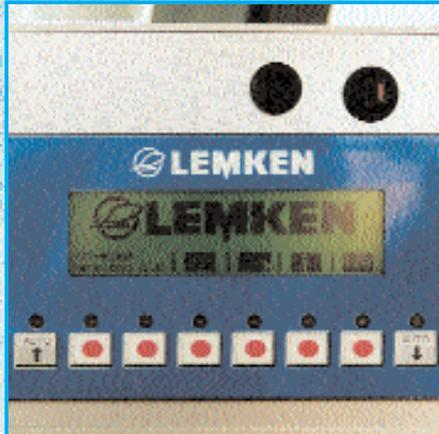
As standard the Titan ploughs are equipped with the electrical turnover control. With this device, the turning and lifting functions is controlled by means of two sensors. The electronic plough control which is available as an option, helps the farmer considerably with its optimal headland management system.
