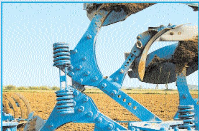
The LEMKEN Non-Stop trip mechanism features short, doubled, coil springs which guarantees high tripping and re-entry forces.
