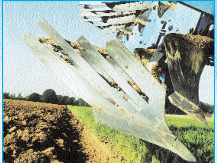
**The shares** comprise separate component plates of micro-alloy boron-steel. Overlapping design avoids roots or other foreign objects being caught. Tight fitting and firm attachment guarantees, wear resistance and reliability against breakage.
