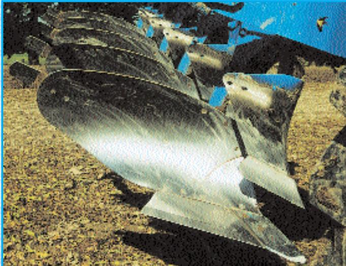
**The plough body** is tempered and thus very strong. Each share is adjustable for pitch and thus always allows a good entry of the plough. The smooth progression from share to mouldboard and the low-resistance offered by the shape of the overall plough body reduce tractive force requirements even more.
