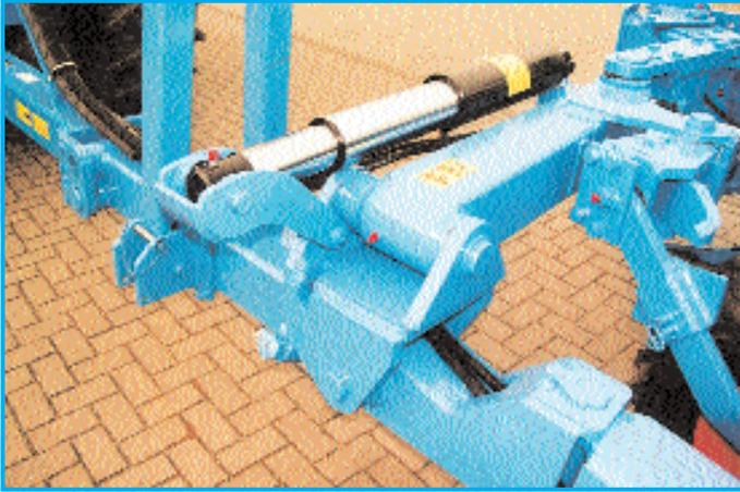
The plough is turned 180° precisely and shock-free by two telescopic cylinders and the smooth operation means required hydraulic working pressure is low. Precise vertical angle settings are per adjuster screws for each side. The robust plough stands mean the plough can be simply detached in transport position and fits compactly into the implement shed.
